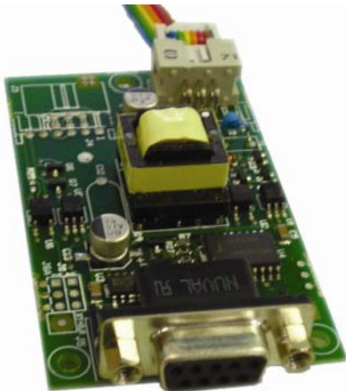
RS-232 communications board
