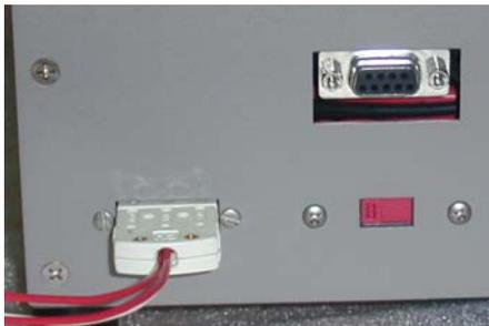
Connect the sensor to the back of the chiller, slide the the selector switch towards the connector, turn the unit on and verify the function and safety.
