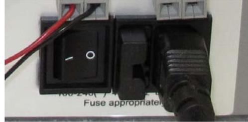
Step 5: Closely observe the operation of the unit. Set the controller to -10. Carefully touch the plate or monitor it's temperature with a separate instrument to insure it's cooling.
