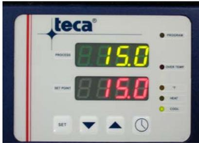
Put something on the cold plate and adjust the set point using the arrow keys.
